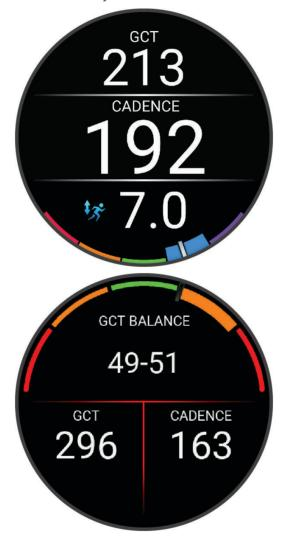
**REMEMBER:** Ground contact time balance is only available if you are using a compatible running dynamics accessory.
